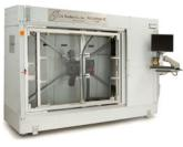
AccuMap-SE<sup>®</sup> Characterize thin film uniformity of large panels with ease. The AccuMap-SE combines a high-speed M-2000 ellipsometer, wide spectral range, and fast mapping for large panels. Perfect for photovoltaic or flat panel display thin films.
