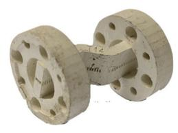
Fig. 12. Manufactured through-type structure for estimating attenuation of test fixture
