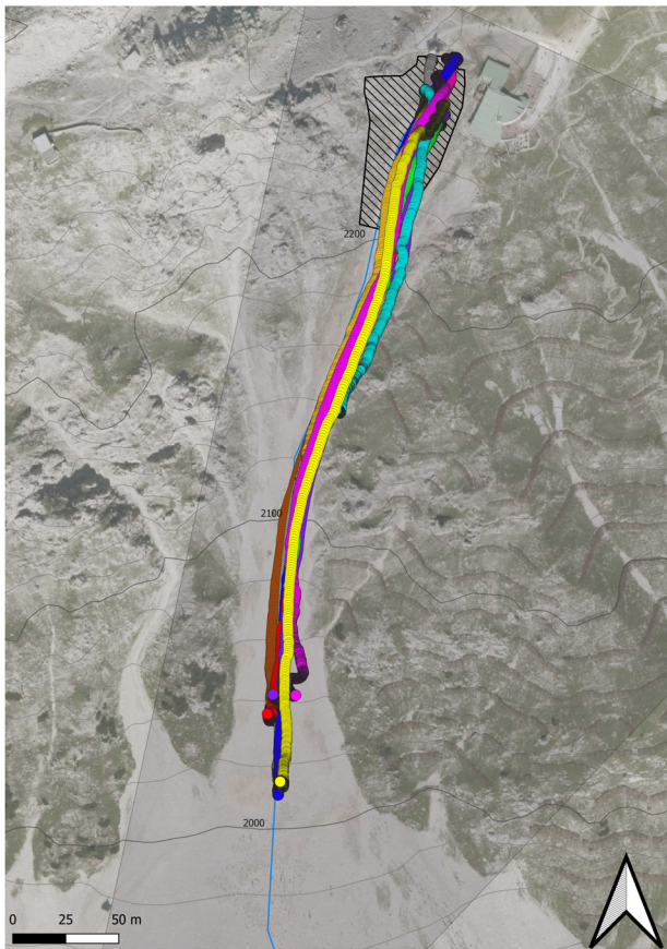
Figure 4. In the left panel, trajectories or GNSS positions of all avalanche experiments are displayed. The spacing of the isochronous sampled position data indicates the flow velocity, e.g. the herein called position velocity v_p . The dot size is set to 5 m, which corresponds to the accuracy stated by the manufacturer. The hatched area represents the release zone. In the right panel the projected travel length \Delta s_{xy}(t) and the altitude difference \Delta Z(t) are shown.
