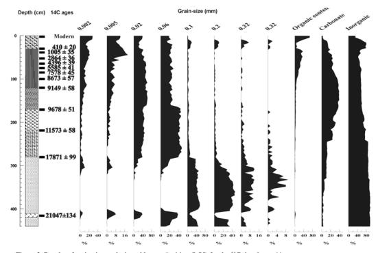
Figure 2 Results of grain-size analysis and loss on ignition (LOI) for the <sup>14</sup>C-dated core 11
