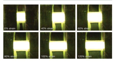
Device characterization of a stretchable polymer light-emitting electrochemical cell. Reproduced with permission from *Nat. Photonics*. **7** (2013), DOI: 10.1038/nphoton.2013.242; p. 817. © 2013 Macmillan Publishers Ltd.
