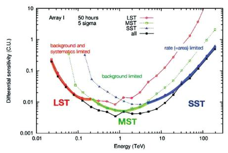
**Figure 9.** The differential sensitivity of CTA configuration "I" and of its LST, MST and SST sub-arrays, showing how the telescopes of different size allow to cover a large spectral range from a few tens of GeV to above 100 TeV (from Bernlohr *et al.* (2012)).
