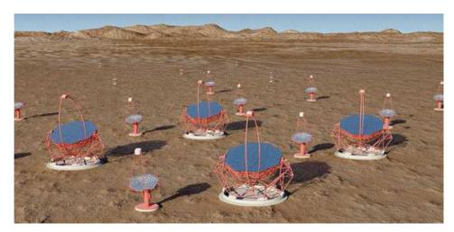
**Figure 7.** Virtual image of the future Cherenkov Telescope Array showing large (LST), medium (MST) and small size (SST) telescopes. One possible configuration for the southern array consists in a low-energy section above a few tens of GeV with four 23 m parabolic telescopes, a core-energy array with twenty-three 12 m Davies-Cotton telescopes in the range 100 GeV to 10 TeV, and a high-energy section with thirty-two 4-6 m Davies-Cotton or Schwarzschild-Couder telescopes at multi TeV energies.
