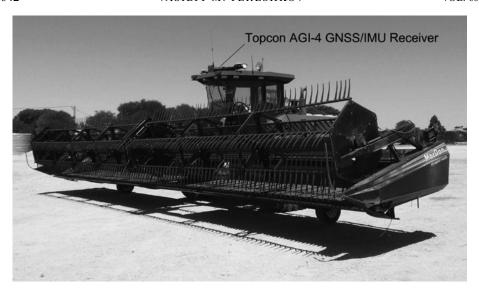
Figure 2. MacDon 9300 Self-Propelled Windrower with Topcon AGI-4 GNSS/IMU Receiver.
