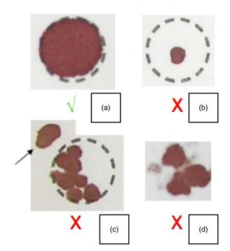
**Fig. 1.** Quality control criteria for dried blood spots from the Food4Me study. (a) Spot suitable for analysis. (b–d): Spots not suitable for analysis due to (b) small spot size not filling the circle, (c) multiple application of too small spots, including spots outside the circle, (d) multiple application of small spots and no thorough soaking of the paper (view from the back).
