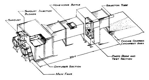
Fig. 1. Schematic drawing of low-speed wind tunnel used to study model precipitation gages under simulated snowstorm conditions
