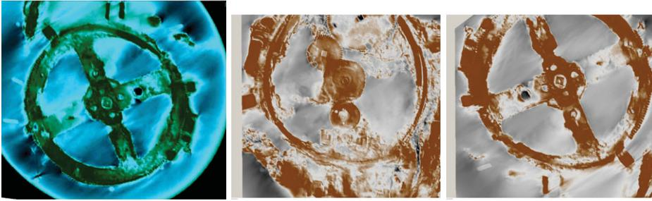
**Figure 1.** Fragment A with the main wheel that drives the Sun and eventually all gears. Images created by the author using X-ray tomography of X-tek raw data and Volume Graphics software.
