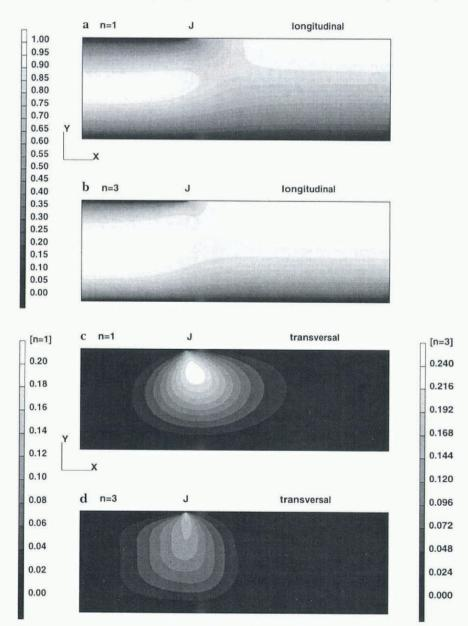
Fig. 5. Numerically calculated velocities for a no-slip/free-slip transition at  $\mathcal{J}$  for n = 1 (a and c) and n = 3 (b and d). General flow direction is from left to right.
