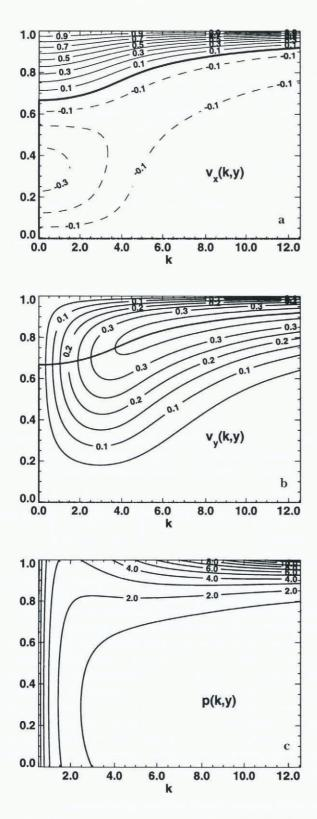
Fig. 3. Square-root power spectrum of the anomalous longitudinal velocity  $v_x(k, y)$  (a), the transversal velocity  $v_y(k, y)$ (b), and the pressure distribution p(k, y) (c).
