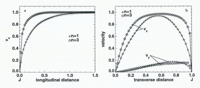
Fig. 4. (a) Longitudinal velocities  $(v_x)$  along the center line as functions of the longitudinal distance from the junction point (J). (b) Longitudinal and transversal velocities along a transverse profile. The velocities are normalized by the maximum longitudinal velocities at the center line. Symbols represent calculated values. Lines are based on linear interpolations.
