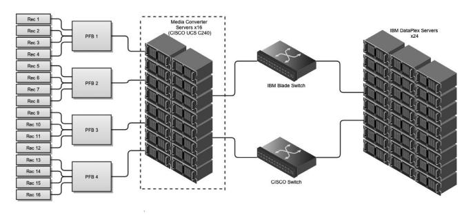
**Figure 1.** Simplified illustration of the MWA digital signal path. For the VCS mode, the baseband data between the fine channel polyphase filter bank (PFB) and the X-engine of the correlator are written to local RAIDs on the 16 media converter servers (highlighted with a dashed box). This gives us 100  $\mu$ s resolution and frequency channels 10 kHz wide.
