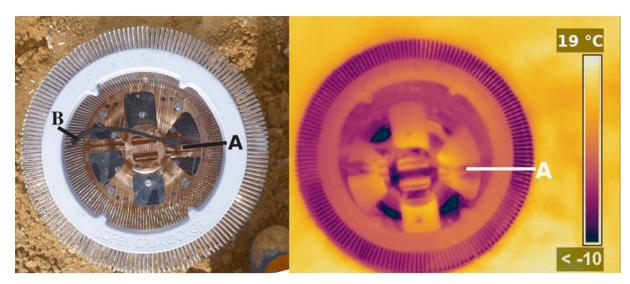
**Fig. 8.** Top view of the Seebeck generator (left) and corresponding image in thermal infrared (right). The heat pipes incorporated into the heat sink assembly (marked A) appear cold, suggesting that they were not operating correctly (note that these heat pipes are distinct from that labelled B in Fig. 1). The atmospheric temperature sensor is marked B.
