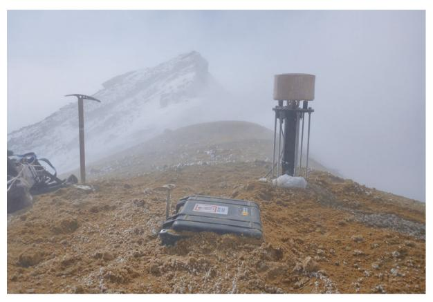
Fig. 4. The Seebeck generator installed in the hot ground. The data logger is housed in the black Peli case.
