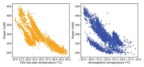
Fig. 6. Scatter plots of thermoelectric generator (TEG) hot-side temperatures (left) and atmospheric temperatures (right) against power output for the time period denoted by the shaded region in Fig. 5. Each data point represents a 1 min average of the recorded values.
