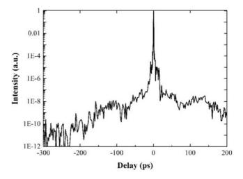
Figure 11. Third-order correlation contrast measurement of the compressed pulse.
