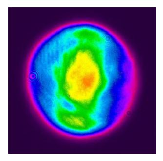
Figure 9. Near-field beam profile of the amplified pulse.
