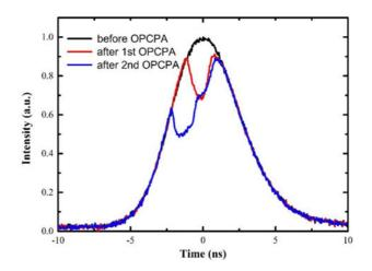
Figure 6. Time profiles of the pump pulse in the OPCPA pre-amplifier.
