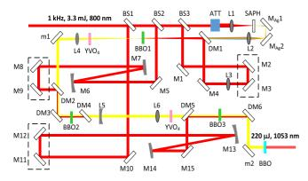
**Figure 2.** Layout of the OPA–SHG pulse cleaning device. BS1–BS3: beam splitter; ATT: attenuator; L1–L6: lens; SAPH: sapphire plate; M<sub>Ag</sub>1, M<sub>Ag</sub>2: silver mirror; DM1–DM6: dichroic mirror; M1–M15: 800 nm HR mirror; m1, m2: 2106 nm HR mirror.
