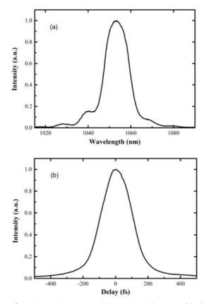
Figure 3. (a) Measured spectrum and (b) autocorrelation trace of the OPA–SHG cleaning pulses.
