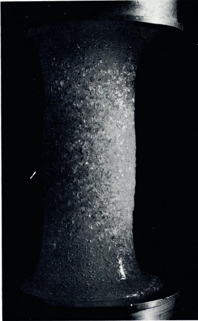
Fig. 15. Dumbbell compression specimen after failure. The center section is filled with internal cracks. At an earlier stage in the deformation, such specimens develop a lumpy surface as surface grains bulge out.
