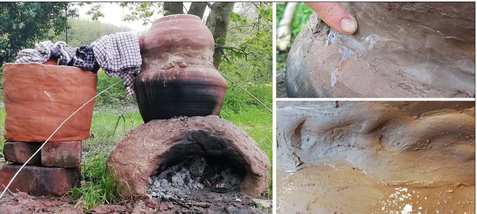
Figure 3. Complete experimental apparatus (left) and distillate leaking through a channel created at a contact point between the still body and head (right) (after Groat 2023: fig. 59).
