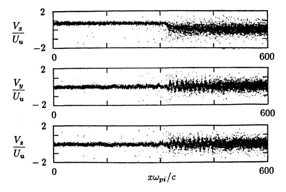
Figure 3. Simulation of a parallel shock by Quest (1987). The shock has an Alfvén Mach number of 5. Distance is measured in units of the ion inertial length (equal to ~ 0.8 thermal ion gyro radii downstream). Note the oscillations in the downstream transverse bulk velocity identifiable as a firehose instability. Also note the backstreaming suprathermal ions ahead of the shock  $(V_X > 0)$ .
