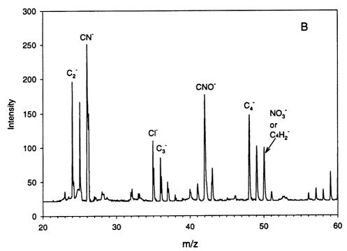
Fig. 3. A. Full LAMMA positive ion time-of-flight spectrum (snow sample from Summit, Greenland). B. LAMMA negative ion time-of-flight spectrum zoomed into the region between 20 and 60 m/z (snow sample from Summit, Greenland). Note that these are not absolute assignments and could be other ions.
