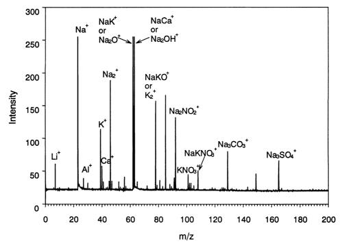
Fig. 2. LAMMA positive ion time-of-flight spectrum (snow sample from Summit, Greenland). Note that these are not absolute assignments and could be other ions.
