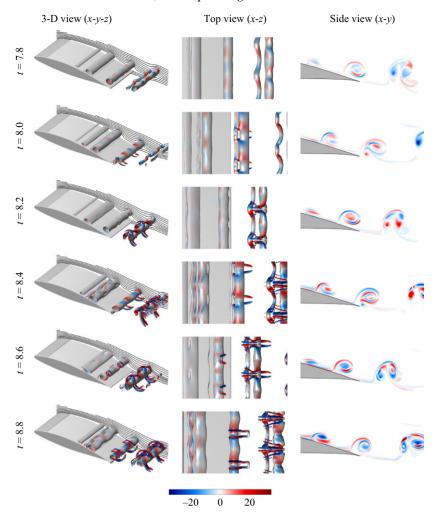
Figure 16. First two columns: iso-surfaces of *Q*-criterion (level: 100) coloured by streamwise vorticity from t = 7.8 to t = 8.8. Instantaneous streamlines in black. Third column: contours of streamwise vorticity  $\omega_x$  at z/c = 0.25. Here,  $\alpha = 7^{\circ}$ .
