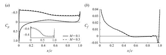
Figure 24. Time-averaged pressure and skin-friction coefficients for M=0.1 and M=0.3 at  $\alpha=4^{\circ}$ , R=30c.
