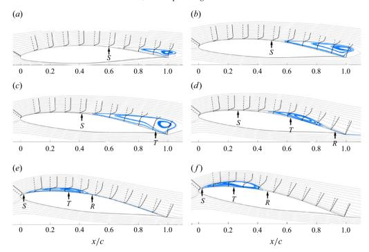
Figure 5. Time- and space-averaged streamlines for  $\alpha$  from  $0^{\circ}$  (a) to  $10^{\circ}$  (f). Recirculating flow in blue. Here, S, T and R indicate the mean locations of separation, transition and reattachment.
