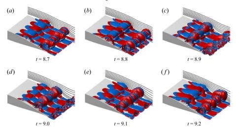
Figure 18. Iso-surfaces of the streamwise vorticity  $+\omega_x$  (red) and  $-\omega_x$  (blue) for a level  $|\omega_x|=1$ . Rear section of the airfoil shown between x/c=0.4 and x/c=1.1 for t=8.7 (a) to t=9.2 (f). Instantaneous streamlines in black. Here,  $\alpha=7^\circ$ .
