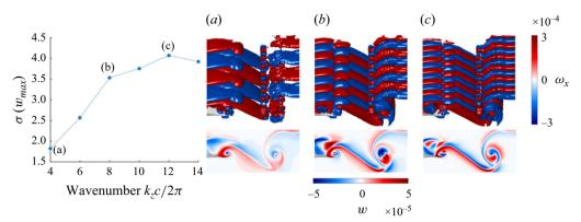
Figure 13. Left: temporal growth rate of  $w_{max}$  for  $\alpha = 6^{\circ}$ . Top right: iso- $\omega_x$  surfaces for wavenumbers 4 (a), 8 (b) and 12 (c) at t = 1.0. Bottom right: corresponding contours of w.
