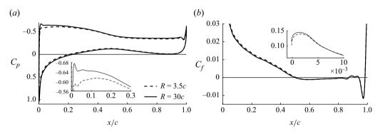
Figure 29. Time-averaged pressure and skin-friction coefficients for R=3.5c and R=30c at  $\alpha=4^{\circ},$  M=0.3.
