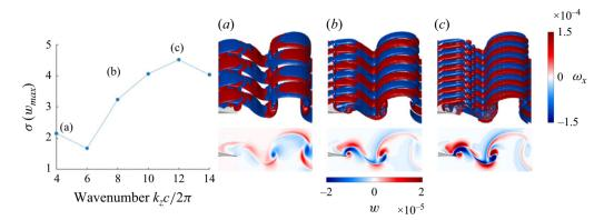
Figure 12. Left: temporal growth rate of  $w_{max}$  for  $\alpha = 4^{\circ}$ . Top right: iso- $\omega_x$  surfaces for wavenumbers 4 (a), 8 (b) and 12 (c) at t = 1.0. Bottom right: corresponding contours of w.
