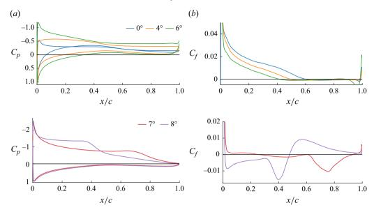
Figure 4. Time- and spanwise-averaged pressure (upper and lower side) and skin-friction (upper side) coefficients for  $\alpha = 0^{\circ}$ ,  $4^{\circ}$ ,  $6^{\circ}$  (top row),  $7^{\circ}$ , and  $8^{\circ}$  (bottom row).
