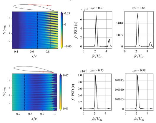
Figure 7. Space–time diagram of the vertical velocity component (v) along the shear layer (left) for  $\alpha = 6^{\circ}$ . The PSD at two locations (indicated by dashed lines) on the right. Top: suction side, bottom: pressure side.
