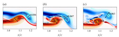
Figure 10. Streamlines of the pressure-side (orange) and suction-side (blue) vortices for  $\alpha = 0^{\circ}$  (a),  $4^{\circ}$  (b) and  $6^{\circ}$  (c). Streamlines are generated by subtracting the velocity at the respective vortex centres. Colouring is by spanwise vorticity  $\omega_z$ .
