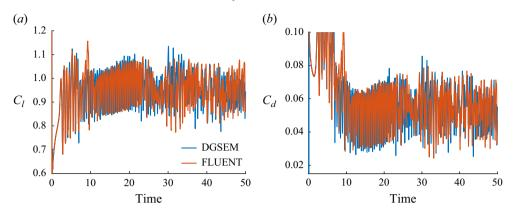
Figure 26. Lift and drag coefficients at  $\alpha=8^{\circ}$  over time DGSEM (M=0.05) and FLUENT (incompressible) computations.
