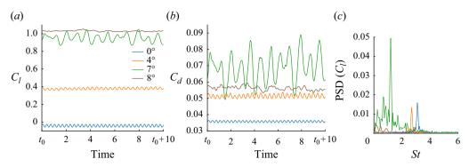
Figure 21. Lift (a) and drag (b) coefficients over time. (c) Frequency spectrum of the lift coefficient. For  $\alpha = 0^{\circ}$ ,  $4^{\circ}$ ,  $7^{\circ}$  and  $8^{\circ}$ .
