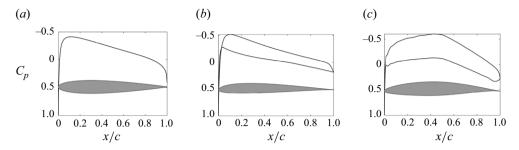
Figure 1. Pressure coefficients (black) for inviscid flow over airfoils (grey) at  $\alpha=0^{\circ}$ . NACA 0012 (a), SD 7003 (b) and NACA 65(1)–412 (c) (Drela 1989). The locations of maximum thickness are at 0.3c, 0.25c and 0.4c, respectively.
