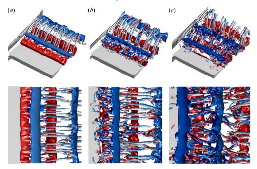
Figure 9. Trailing-edge view of iso-Q surfaces for  $\alpha = 0^{\circ}$  (a),  $4^{\circ}$  (b) and  $6^{\circ}$  (c). Colouring is by spanwise vorticity  $\omega_z$ .
