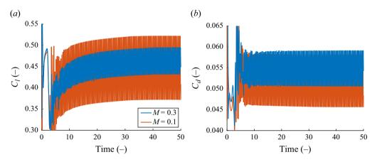
Figure 23. Lift and drag coefficients at  $\alpha = 4^{\circ}$  over time for different Mach numbers. Domain radius R = 30c.
