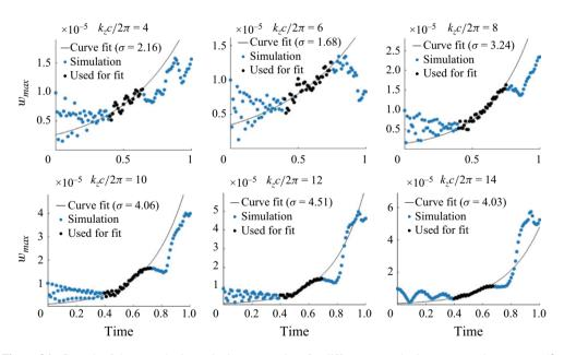
Figure 34. Growth of the perturbation velocity w over time for different perturbation wavenumbers at  $\alpha = 4^{\circ}$ .
