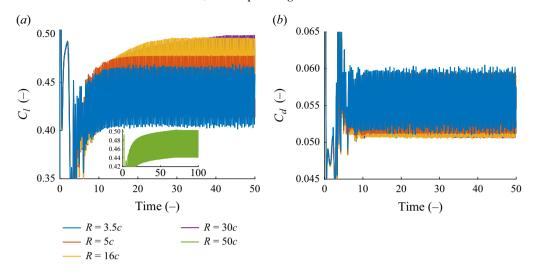
Figure 28. Lift and drag coefficients over time for different computational domain sizes and  $\alpha = 4^{\circ}$ , M = 0.3.
