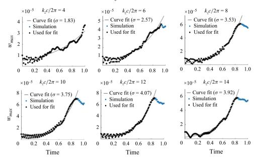
Figure 35. Growth of the perturbation velocity w over time for different perturbation wavenumbers at  $\alpha = 6^{\circ}$ .
