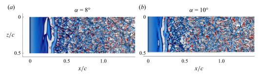
Figure 20. Iso-Q surfaces for  $\alpha = 8^{\circ}$  (a) and  $10^{\circ}$ . Colouring by spanwise vorticity  $\omega_z$ .
