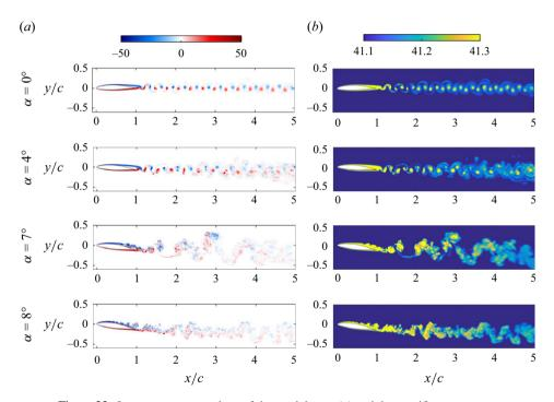
Figure 22. Instantaneous snapshots of the vorticity  $\omega_z$  (a) and the specific entropy  $s=\ln(p/\rho^\gamma)/(\gamma(\gamma-1)M_f^2)$  (b) along a slice at z/c=0.025 for  $\alpha=0^\circ,4^\circ,7^\circ$  and  $8^\circ$  (top to bottom).
