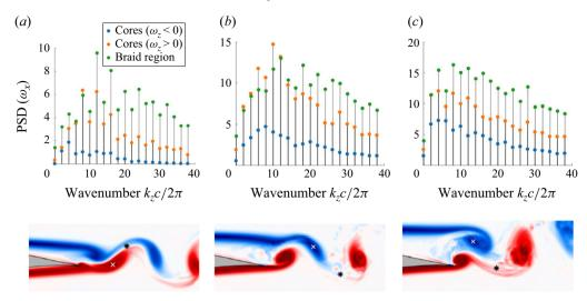
Figure 11. The PSD of the spanwise vorticity  $\omega_z$  along the span for the vortex cores and the braid region located downstream of evaluated core. Bottom row: snapshots of spanwise-averaged  $\omega_z$  contours with vortex cores (white  $\times$ ) and braid location (black \*).
