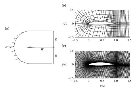
Figure 2. (a) A C-type computational domain with general parameters. Elements of 2-D computational meshes for *grid* 1 (b) and *grid* 2 (c) around the airfoil. Only elements without interior Gauss nodes are shown.
