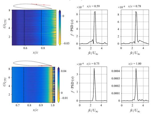
Figure 8. Space–time diagram of the lateral velocity component (v) along the shear layer (left) for  $\alpha = 4^{\circ}$ . The PSD at two locations (indicated by dashed lines) on the right. Top: suction side, bottom: pressure side.
