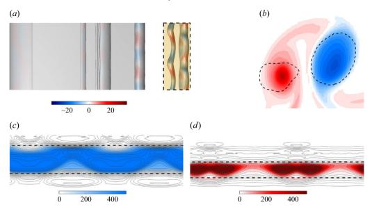
Figure 17. (a) Top view (x-z) of Q-criterion isosurfaces coloured by streamwise vorticity with highlighted vortex pair in near wake. (b) Side view (x-y) of spanwise vorticity contours of the highlighted vortex pair. Dashed lines indicated spanwise-averaged iso-Q contours. (c-d) Front view (z-y) of a slice through the vortex pair (c)  $\omega_z < 0$ , (d)  $\omega_z > 0$ . Dashed lines are spanwise-averaged iso-lines of Q (level: 8). Here,  $\alpha = 7^\circ$  at t = 7.8.
