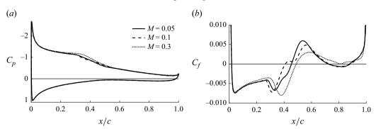
Figure 25. Time-averaged pressure and skin-friction coefficients for different Mach numbers at  $\alpha = 8^{\circ}$ , R = 30c.
