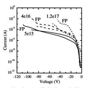
Fig. 15. Breakdown characteristics of diodes under reverse bias [9].
