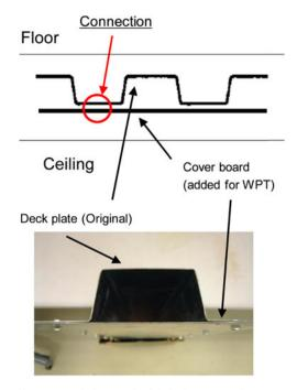
Fig. 3. Illustration and photograph of deck plate waveguide.
