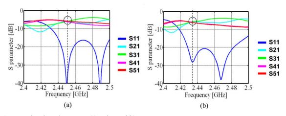
Fig. 10. S parameters for each port shown in Fig. 9: (a) simulation and (b) measurement.
