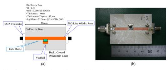
Fig. 16. GaN diode rectifier of  $V_{br} = 100$  V and ten fingers: (a) illustration and (b) photograph.
