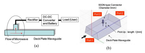
Fig. 7. (a) Block diagram of the rectenna outlet, (b) detail of the microwave pick-up.
