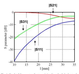
Fig. 8. Simulated S parameters for transmission from the deck plate to the coaxial pick-up.
