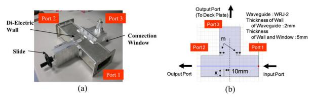
Fig. 5. (a) Photograph and (b) illustration of the developed power divider.
