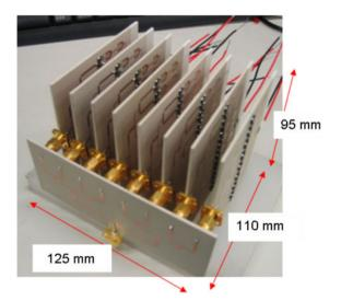
Fig. 11. Developed 64-divided high-power rectenna composed of 256 Si Schottky barrier diodes.
