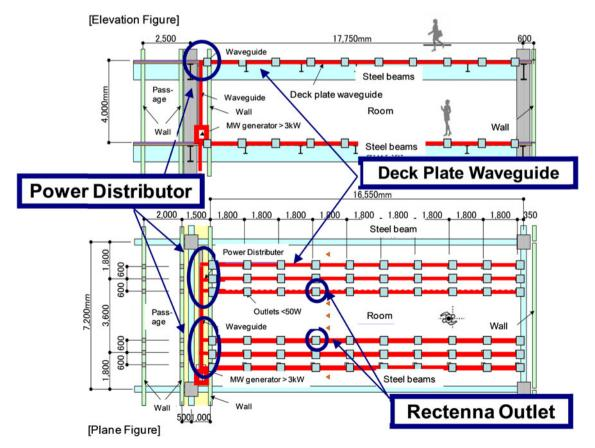
Fig. 2. Elevation and plane diagrams of the WPDS.
