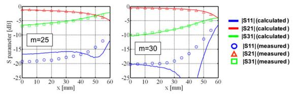
Fig. 6. Simulated and measured  $S_{11}$ ,  $S_{21}$ , and  $S_{31}$  with x and m parameters.
