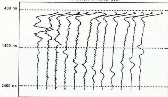
Fig. 4. An ice-radar profile across Mount Estelle glacier as recorded using the PC-based receiver.
