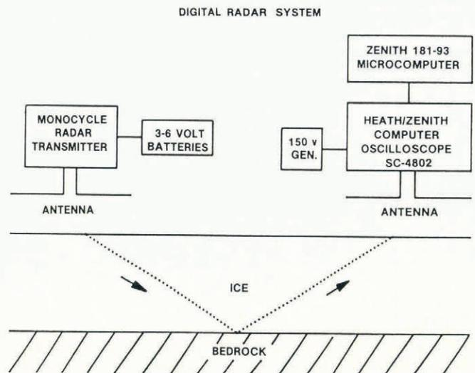
Fig. 2. Block diagram of an ice-radar system including the PC-based receiver.
