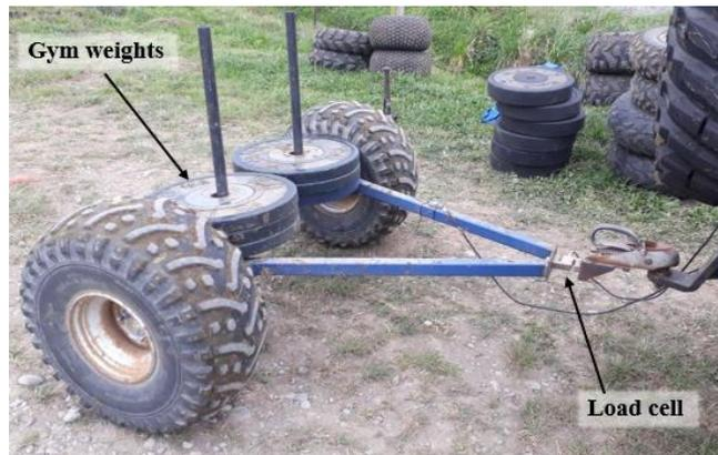
Figure 3. Towed test rig
