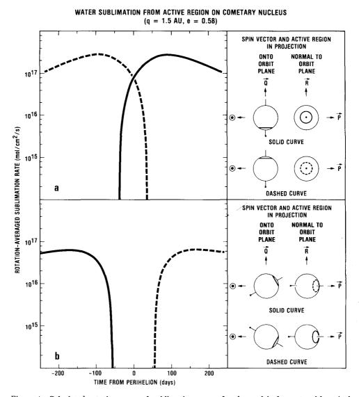
Figure 4. Calculated rotation-averaged sublimation curves for the nuclei of comets with a single active region on the surface. The parameters  $\Phi$ , I, and  $\phi$  for the solid/dashed curves are: 0°, 90°,  $+60^{\circ}/-60^{\circ}$  for panel *a* and  $60^{\circ}/120^{\circ}$ ,  $90^{\circ}$ ,  $-60^{\circ}$  for panel *b*. See the caption to Fig. 2 for further information.
