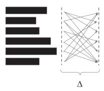
Fig. 1. bsp system computation model. Each node's computation is independent but bounded by the global end of the round (condition S2). Communication is reliable and takes exactly  $\Delta$  time (conditions S3 and S3'). The next round starts when  $\Delta$  time since the end of the previous round has elapsed (conditions S1 and S3').
