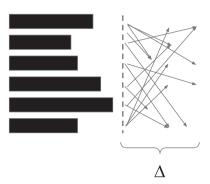
Fig. 4. bsp-d system computation model. Differently than *bsp* systems, the next round starts right after the end of the current one. Additionally, data communication may take arbitrary (although bounded) time.
