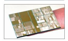
One of the nanotechnology-inspired grand challenges suggested by the White House is to create computer chips that are 100 times faster yet consume less power. This picture shows a computer chip with 7-nm transistors that IBM made by using silicongermanium instead of silicon. The technology could enable up to 20 billion transistors on a fingernail-sized chip. Credit: Darryl Bautista/Feature Photo Service/IBM.
