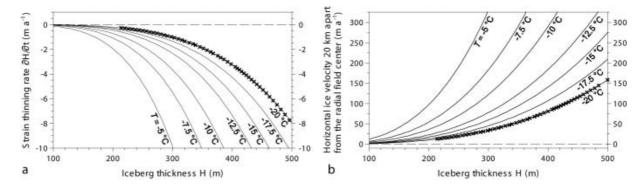
**Fig. 3.** (a) Variation of strain thinning rate  $\partial H/\partial t$  with thickness H and temperature T of a rectangular isothermal iceberg with constant density (915 kg m<sup>-3</sup>), based on analytical calculations of Equation (10); crosses indicate results from a time-dependent application of the iceberg model. (b) Corresponding diagram of horizontal ice velocity 20 km from the radial field center vs iceberg thickness and temperature, based on Equation (11).
