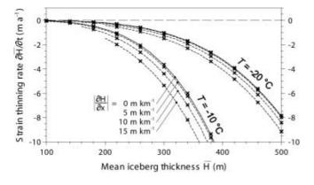
**Fig. 4.** Variation of strain thinning rate  $\partial \bar{H}/\partial t$  with mean iceberg thickness  $\bar{H}$  for different ice temperatures and longitudinal thickness gradients  $\partial H/\partial x$ . Model results (dashed curves and crosses) obtained for an idealized isothermal iceberg of constant density (915 kg m<sup>-3</sup>) match the curves for  $\partial H/\partial x=0$  which are derived from analytical calculations of Equation (10).
