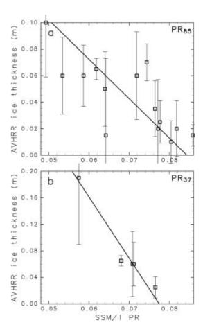
**Fig. 6.** Scatter plot of the AVHRR ice thickness vs SSM/I PR for (a) 85 GHz and (b) 37 GHz. The solid line denotes the principal-component axis of these plots. The vertical lines with crossbars show the standard deviation of AVHRR ice thicknesses in the SSM/I gridcell in each plot.
