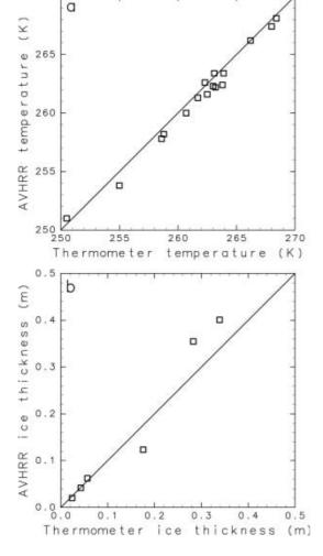
**Fig. 3.** Scatter plots of (a) the AVHRR temperature vs thermometer temperature; and (b) the AVHRR ice thickness vs the thermometer ice thickness.
