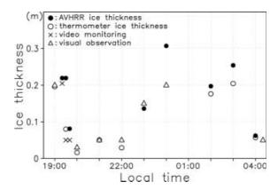
**Fig. 4.** Comparison of sea-ice thickness derived from several methods along the cruise track in the Vincennes Bay polynya during the night-time, with the abscissa being local time.
