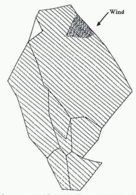
Fig. 5. An example of analysis. The very shaded surface is the small panel that acts as the trigger. The shaded surface is the part of starting zone which is released, the white surfaces are the part which is not released. Lines are boundaries of large panels. The trigger is just beside the upper ridge because the east wind creates a large accumulation of snow there.
