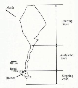
Fig. 2. Ciagé Valley in Tende near Nice. Some of the houses must be protected from an avalanche. This article deals with an analysis of the starting zone with a knowledge-based system. On the avalanche track and the stopping zone, numerical models can be used.
