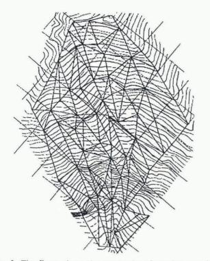
Fig. 3. The figure shows the topography of starting zone in Ciagé Valley and the triangular irregular grid used as digital terrain model.
