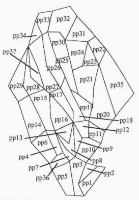
Fig. 4. This figure shows the partition of starting zone in small panels. Each small panel is almost homogeneous from the point of view of slope, vegetation, exposure and distance to ridges. Ridges are not represented here.
