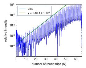
**Figure 5.** Measurement of the relative pulse energy as a function of the number of round trips in the regenerative amplifier. The part when  $N \in [20...40]$  is used for the fit.
