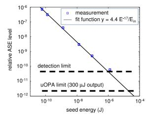
**Figure 4.** ASE level at PHELIX as a function of the seed energy measured at the regenerative amplifier stage input.
