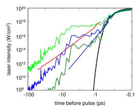
**Figure 6.** Comparison of the single (blue) and double (dark green) plasma mirror effect to the plasma expansion threshold for gold (red) and hydrogen (blue).
