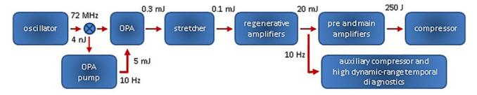
Figure 3. Schematics of the low-ASE version of the PHELIX laser commissioned in 2012. The auxiliary compressor is used for temporal contrast characterization on a daily basis.
