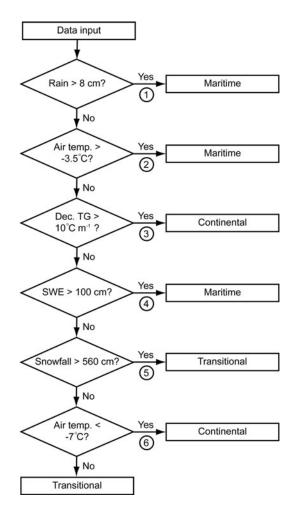
**Fig. 3.** Flow chart illustrating the classification procedure for the seasonal snow-climate classification (after Mock and Birkeland, 2000). SWE: snow water equivalent, TG: temperature gradient.
