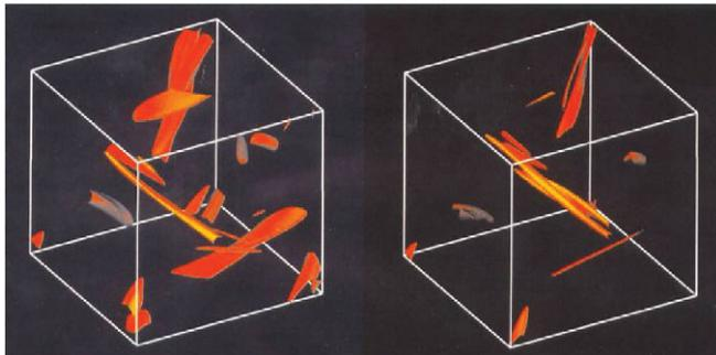
**Figure 1.** The *ABC* dynamo with (1,1,1) forcing, for  $\nu = 1/5$ ,  $\eta = 1/400$ . Shown are isosurfaces where the magnetic energy attains 20% of its maximum value at that instant, for two separate times approximately 40 turnover units apart.
