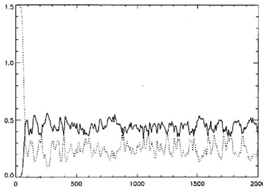
**Figure 2.** The same case as in Figure 1, but now showing the evolution of total magnetic energy (solid) and total kinetic energy (dashed), for a time long compared with the turnover and both diffusion timescales.
