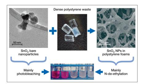
Schematic describing preparation of  $SnO_2$ -polystyrene (PS) nanofoams from waste PS leading to a porous material, and the two main photochemical mechanisms observed for photocatalytic degradation of RhB, photobleaching (using  $SnO_2$  alone), and N-de-ethylation (using  $SnO_2$ -PS nanofoams). Credit: Rodrigo J. de Oliveira.
