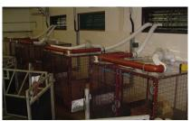
Figure 1 Chambers to measure methane emission from small ruminant
