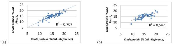
**Figure 1** Regression of crude protein content (% DM) quantified with Phazir spectrometers against crude protein content quantified with reference method (Foss NIR 5000). (a) Phazir 1624 - (b) Phazir 1018
