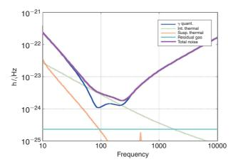
Figure 4 Predicted sensitivity spectrum for Advanced LIGO.
