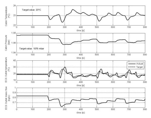
Figure 3. Simulation results: cabin and ECS outputs.
