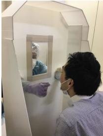
Fig. 1. The photo shows the healthcare worker (HCW) and patient sides of the shield. An acrylic plate is used for the window so that the patient's face can be seen clearly. The HCW wears PPE for examinations but does not need to change PPE for each patient. The disposable gloves used for testing must be changed for each patient.
