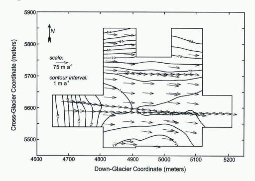
Fig. 2. Velocity field. Vectors show the measured displacement of 110 velocity markers during the period early May to mid-August. Contours are of velocity in m year<sup>-1</sup>. The glacier's approximate center line is the east—west arm located at y = 5600. Velocities are highest along the center line and decrease toward the valley walls. A strong gradient in velocity is present along the western arm of the center line at the base of the upper icefall.
