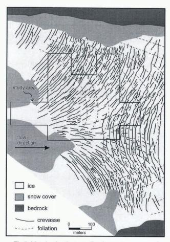
Fig. 7. Map showing the traces of major crevasses as mapped from a vertical air photograph. Digital enhancement of the photograph was used to highlight lineations representing crevasses.
