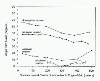
Fig. 8. Observed and calculated rotation. Plot shows the angle between the strike of crevasses and the x axis at an up-glacier and down-glacier transect. Up-glacier is x=4810; down-glacier is x=5100. Observed rotation is difference between the two transects. Calculated rotation is shown with error bars representing upper and lower limit values.
