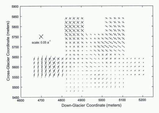
Fig. 5. Axes of principal strain rate plotted to show magnitude and orientation. Values are calculated at the nodes of a  $20 \, m \times 20 \, m$  orthogonal grid.
