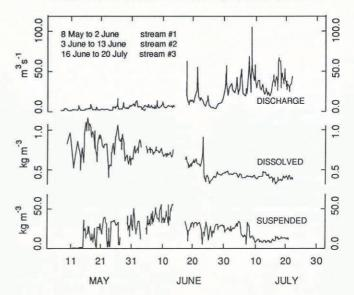
Fig. 5. Manual measurements from the outlet streams during 1983. The time period from 8 May to 20 July encompasses the peak of the surge motion. The surge stopped on 4-5 July.
