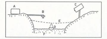
Fig. 2. Sketch of the automatic sensor system in use in 1983: A, recorder; B, acoustic water-stage sensor; C, automatic camera; D, floating instrument package, with turbidity and conductivity sensors; E, cross-stream cable; F, stream.
