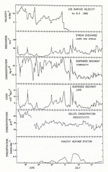
Fig. 6. Measurements from stream #3 during 1983: a. Surface ice velocity at Km9.5 (from Kamb and others, 1985); b. Water discharge estimated by observer; c. Hand measurements of turbidity, converted to suspended-sediment concentration; d. Suspended-sediment load; e. Dissolvedsediment concentration, from hand measurements of electrical resistivity; f. Precipitation at Yakutat weather station (~60 km from the glacier).
