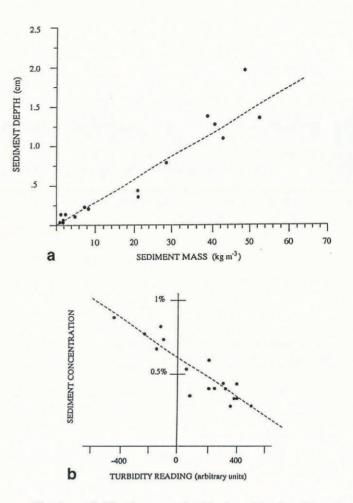
Fig. 3. a. Calibration curve for 21 ml samples (mostly 1983–84 samples). Data from dried and weighed water samples. The water depth in the samples was 13 cm; the line is fitted by eye. b. Calibration curve for August– September 1983 turbidity data from the hand-held instrument. The sediment concentration is expressed as percentage volume, obtained from concurrent water samples.
