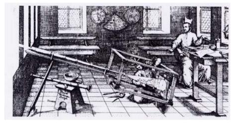
Figure 3. Father Christoph Scheiner (1575 – 1650) using a refracting telescope to project a solar image into an opaque screen. His assistant is apparently marking the positions of sunspots. This image was used as the basis of the Ford Madox Brown painting of William Crabtree observing the 1639 transit.
