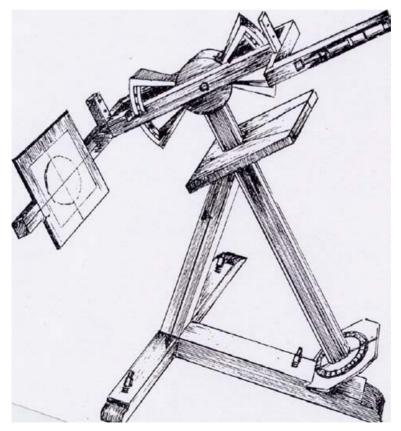
**Figure 4.** The Scheiner helioscope (see *Rosa Ursina* 1630) follows a principle introduced by Tycho Brahe and rotates about a polar axis. A reversed representation of this pioneering equatorial projection telescope was used in the Eyre Crowe (1824 - 1910) painting of Horrocks observing the transit, even though Horrocks probably used a system similar to that used by Crabtree.
