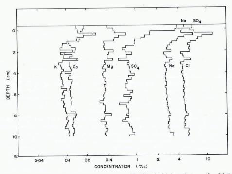
Fig. 1. Ion concentration profiles for saline ice grown at  $-30^{\circ}C$ . (Zero depth indicates the true surface of the ice.)
