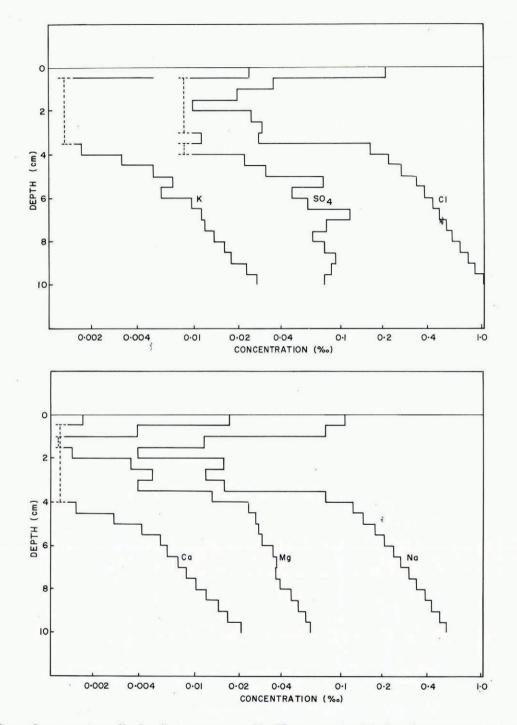
Fig. 3. Ion concentration profiles for saline ice grown at  $-15^{\circ}C$ . (The top 4 cm showed the clear, glassy structure of fresh ice.)
