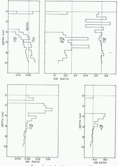
Fig. 4. Ion ratios for saline ice grown at  $-15^{\circ}C$ .
