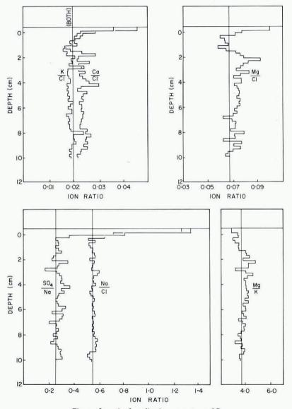
Fig. 2. Ion ratios for saline ice grown at  $-30^{\circ}C$ .
