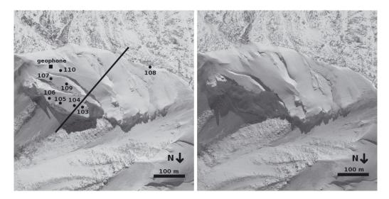
**Fig. 8.** Orthophotograph of Weisshorn glacier on 16 March 2005 (left; before the break-off) and on 3 April 2005 (right; after the break-off) (Swisstopo). The monitored points (black dots) and the geophone (black square) on the east face of the Weisshorn are highlighted. The black line indicates the location of the cross-sectional view (Fig. 9).
