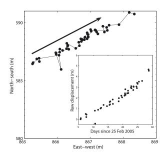
**Fig. 10.** Position of point 103 before correction, projected on the horizontal plane. The arrow indicates the direction of motion. The inset shows the raw displacement before correction as a function of time. This inset can be compared with the displacement after correction (Fig. 11).
