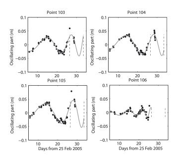
**Fig. 14.** Oscillating part of the four points showing a dramatic acceleration. The solid grey lines indicate the fit of the log-periodic oscillations with parameters of Table 1. The two vertical dashed lines represent the two successive break-off events which occurred on the Weisshorn glacier (after 26.5 and 33.5 days of monitoring). See Figure 8 for point location.
