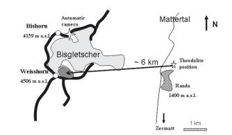
**Fig. 2.** General schematic view of Weisshorn hanging glacier (dashed zone) and the monitoring setting (theodolite and automatic camera). Thick black lines indicate the mountain ridges, and the thin line represents the bottom of the valley.
