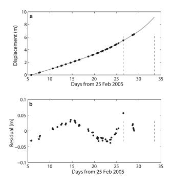
**Fig. 13.** (a) Corrected displacement of Weisshorn glacier at point 103. The grey curve represents the power-law fit (time integral of Equation (1)). (b) Residual of the power-law fit. The two vertical dashed lines show the two successive break-offs (after 26.5 and 33.5 days of monitoring).
