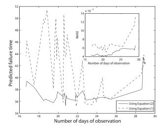
**Fig. 22.** Predicted failure time as a function of the number of days of observation for the Weisshorn 2005 break-off. The dashed curve shows the prediction obtained by fitting Equation (1) and the solid curve the prediction obtained by fitting Equation (2). The inset shows the corresponding RMSE.
