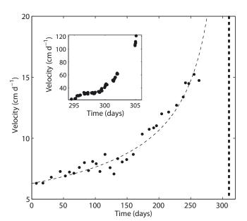
**Fig. 5.** Velocity of Weisshorn glacier before the 1973 break-off. The vertical thick dashed line represents the observed time of failure (at day 306). The thin dashed curve is a fit of the data with Equation (1). The inset shows extensometer measurements a few days before break-off.
