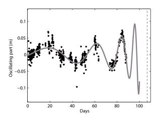
**Fig. 19.** Oscillating part of one measured point on Mönch hanging glacier. Solid line indicates the fit of the log-periodic oscillations. The dashed vertical line shows the break-off occurrence after 107 days of measurements.
