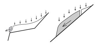
**Fig. 4.** Sketch of Mönch (left; wedge fracture) and Weisshorn (right; slab fracture) break-off. The unstable ice masses are depicted in grey. The mass-balance regime is indicated with arrows (after Pralong and Funk, 2006).
