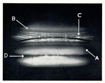
Fig. 2. Side view of the ice dome A, growing between glass plates. There is also a reflection B of the ice in the top plate. Note the smoothness of the ice surface and air bubbles C in the region of contact. The base of the ice is at D.
