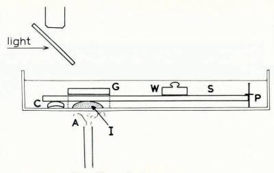
Fig. 1. The crystallization pressure apparatus.
