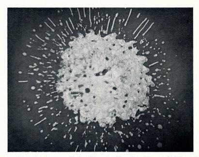
Fig. 3. Appearance of the ice dome in contact with glass slide as viewed from above. Diameter of bright central region approximately 8 mm.
