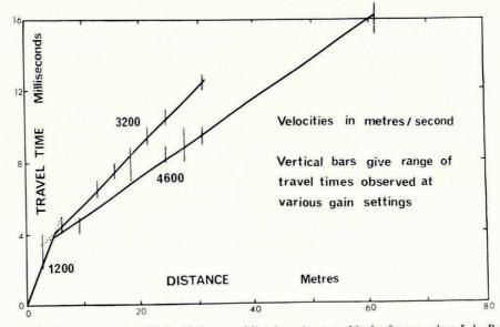
Fig. 5. Seismic travel-time data, Taylor Valley, on exfoliated granite at an altitude of 250 m. above Lake Bonney
