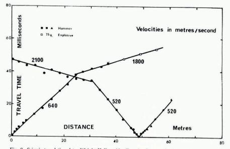
Fig. 8. Seismic travel-time data, Wright Valley, ridge E on ice-free moraine (see Figure 2 and text)
