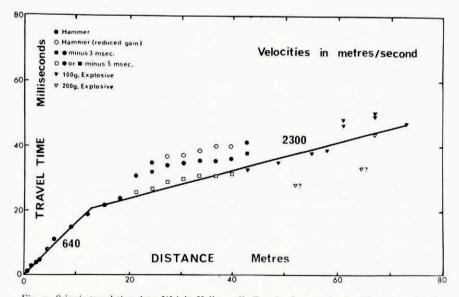
Fig. 9. Seismic travel-time data, Wright Valley, gully F on ice-free moraine (see Figure 2 and text)
