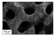
Figure 1. Surface of coral containing interconnected macropores of 150-500 µm.
