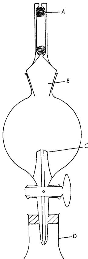
Fig. 1. Inoculation device. *A*, glass tube, packed with non-absorbent cotton wool and joined to a ground-glass stopper *B*. The raised outlet *C* of the separating funnel is designed to ensure that only motile organisms are transferred. *D* is a glass cone, which acts as a shield and locates the neck of the bottle below the delivery tip.
