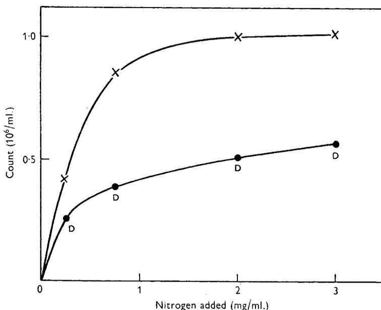
Fig. 2. Effect of oxygen limitation on the growth of *T. pyriformis* on 'vitamin-free' casein for 4 days.  $\times$ — $\times$ , bottles with loose caps;  $\bullet$ — $\bullet$ , bottles with tight caps; D, dead organisms present.
