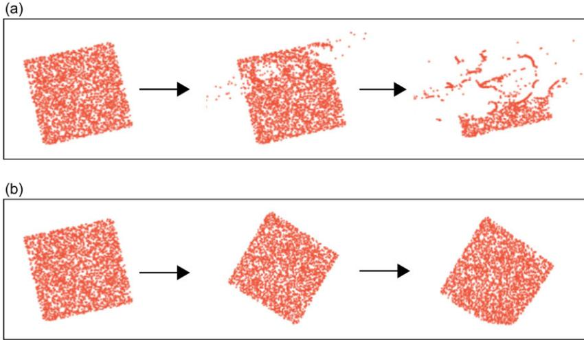
**Figure 3.** The difference of explicit and implicit time frameworks’ simulation results: (a) MPM using explicit framework fails when the simulation with large time step and large material parameters. (b) MPM using implicit framework and automatic differentiation improves the robustness of simulation.
