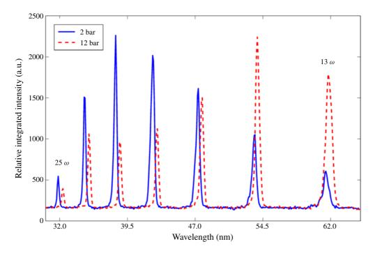
Figure 7. Harmonic spectra from Xe at  $6.5 \times 10^{13}$  W cm<sup>-2</sup> intensity for 2 and 12 bar (dotted line) backing pressure.
