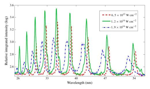
Figure 6. Increasing blue shift of high harmonics with increasing intensity for 12 bar Ar backing pressure.
