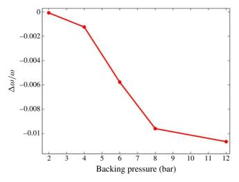
**Figure 8.** Red shift of the 21st harmonic for Xe at  $6.5 \times 10^{13}~\rm W~cm^{-2}$  intensity with increasing pressure.
