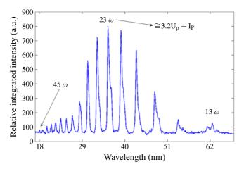
**Figure 2.** The HHG spectrum from Ar at 14 bar backing pressure and  $10^{14}~\rm W~cm^{-2}$  intensity.
