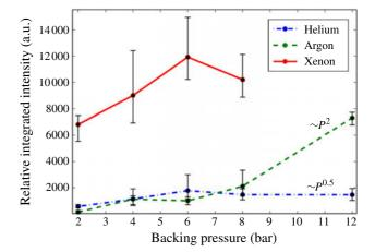
**Figure 4.** Comparison of the pressure dependence of the 25th harmonic at  $6.5 \times 10^{13}$  W cm<sup>-2</sup> intensity in He, Ar, and Xe.
