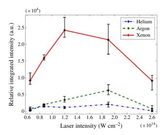
**Figure 3.** Intensity dependence of the 15th harmonic for different gases at 6 bar backing pressure.
