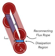
FIGURE 1. Sketch of two reconnecting flux ropes in red with reconnecting magnetic field lines in white. The flux rope radius R and out-of-plane extent  $L_{ext}$  are shown. The dissipation region of thickness  $\delta$  and length L is in blue. The white surface of area A denotes the location of the magnetic field that reconnects in a time  $\Delta t$ .
