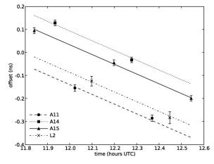
Figure 1. APOLLO residuals from the DE421 ephemeris on the night of 2008 September 24. 0.1 ns in the round-trip time is equivalent to 15 mm of one-way range. A common slope offset applies to all reflectors, indicating a likely earth orientation offset. The separation of the four reflectors is due to imperfect prediction of lunar orientation.
