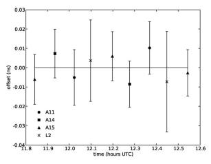
**Figure 2.** Residuals from Fig. 1 after subtracting the individual fit-lines for each reflector. The remaining offsets are artificially small with relation to the error bars because five degrees of freedom have been removed from 9 points (a common slope and four individually-adjusted offsets). Each vertical tick of 0.01 ns corresponds to 1.5 mm in one-way range.
