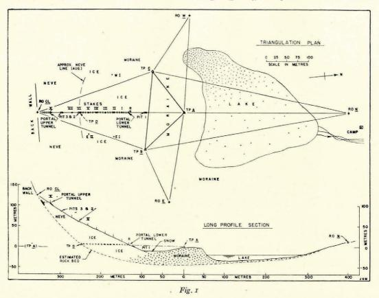
roof peg relative to the line of sight between D and A gave the control basis for all interior measurements. This precise control was necessary because of the small movements, a condition which is in our favour, for one can therefore expect no catastrophic distortion of the tunnel prior to the completion of the year's programme.
